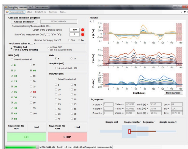
Fig. 1. Measurement window of MAGNUS with: on the right hand side the data progressively acquired and on the left the parameters of the undergoing treatment (e.g. core label, measured steps).
