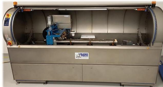
Core scanner XRF
